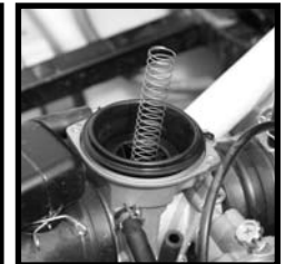
Remove the spring. Do not stretch or bend the spring.
