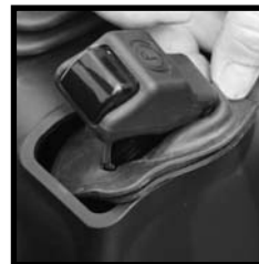
Re-seal the rubber gaskets around the components on the console.
