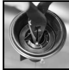
Using long-nose pliers, gently grasp and remove the needle keeper.
