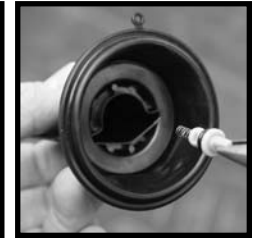
Place the needle back into the diaphragm and reinsert the needle keeper as shown.
