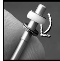
Remove the needle. Take the shim that is sitting on top and move it as shown.
